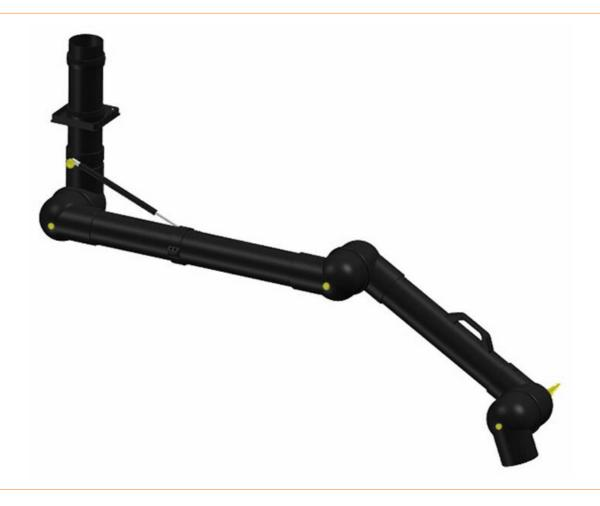
The Alsident DN 100 extraction system is particularly suitable for larger quantities of pollutants or larger collection tasks. The pipes have a diameter of 100 mm and the recommended air volume for the extraction is between 140 m $^3$ /h and 400 m $^3$ /h. The ESD system is supplied with a ground wire with a 1M $\Omega$  resistor.
