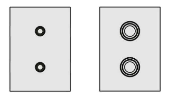
Two coupling sockets in sizes 3 or 4, each with a diameter of 100 mm, are available for an efficient compressed air connection. These enable a reliable connection and optimum compressed air supply for various applications. The standardized sizes ensure easy handling and compatibility in different industrial environments.
