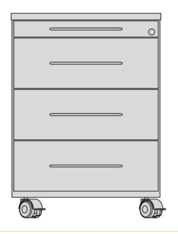
The ESD roll container from Karl consists of a wooden body with 4 drawers, which are equipped with a pull-out safety device. This means that only one drawer can be opened at a time.
