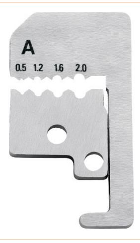
1 pair of spare blades for 12 11 180 With interchangeable blades for four (matched to diameter) or six (matched to cross-section) different conductor cross-sections. No damage to the conductor due to precisely ground form blades, even fine stranded wires are stripped gently. Clamping jaws hold the wire firmly during stripping. With adjustable length stop for equal stripping lengths when working in series. A pressure spring returns the pliers to their original position.
