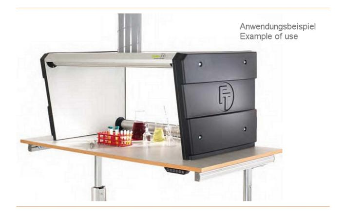
• The CBC-A extraction cabinet with air barrier has a unique ventilation concept that separates the user from the application by means of a double air barrier with unrestricted access to the workbench. The cabinet is located directly on the workbench and can be connected to a central extraction system via the 160 mm connection. Required minimum fume cupboard volume: 180 m<sup>3</sup>/h. Maximum suction volume: 230 m<sup>3</sup>/h.
