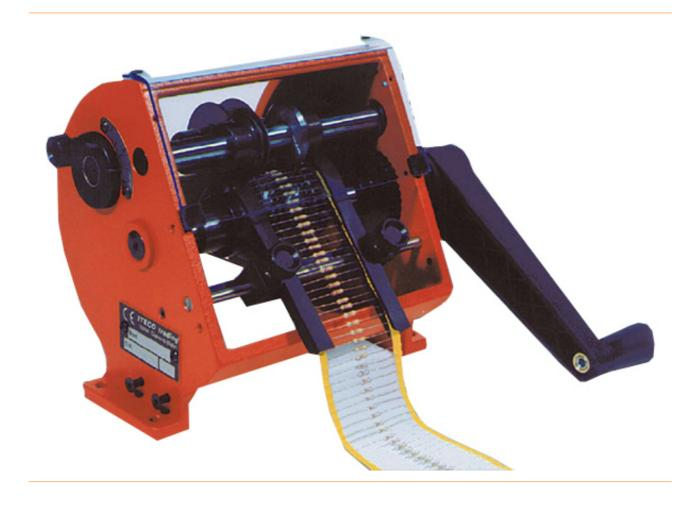
Bending and cutting device for cutting, bending, crimping of axially taped components
