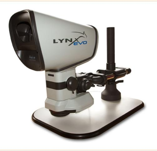
The eyepieceless stereo microscope allows a 3-dimensional image representation in firstclass quality in a comfortable working position. The Lynx EVO is an ergonomically designed stereo microscope and does not require any adjustment by the operator. With the zoom factor 10:1 the magnification of 6x - 60x can be increased to 120x with additional lenses. Optionally, a camera package can be added, which allows seamless image/video storage.
