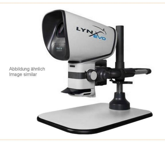
The eyepieceless stereo microscope allows a 3-dimensional image representation in firstclass quality in a comfortable working position. The Lynx EVO is an ergonomically designed stereo microscope and does not require any adjustment by the operator. With the zoom factor 10:1 the magnification of 6x - 60x can be increased to 120x with additional lenses. Optionally, a camera package can be added, which allows seamless image/video storage.
