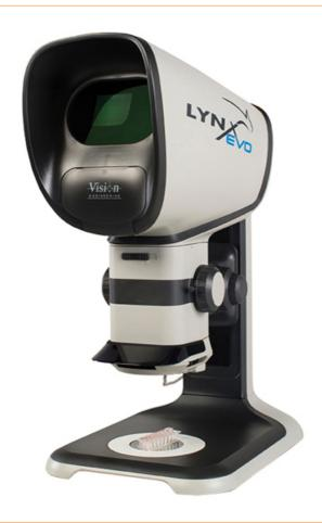
The eyepieceless stereo microscope allows a 3-dimensional image representation in firstclass quality in a comfortable working position. The Lynx EVO is an ergonomically designed stereo microscope and does not require any adjustment by the operator. With the zoom factor 10:1 the magnification of 6x - 60x can be increased to 120x with additional lenses. Optionally, a camera package can be added, which allows seamless image/video storage.
