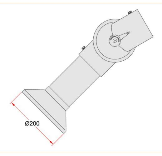
Metal hood recommended for detection of hot gas, smoke and light dust quantities
