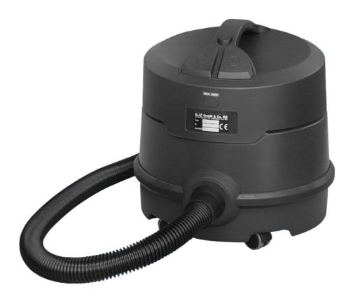
The ESD vacuum cleaner EPA-VAC is suitable for use in ESD protection zones (EPA). It has a low-noise motor and enables extremely quiet vacuuming with 54 dB at the lowest level. The ESD vacuum cleaner consists of black polypropylene, which is permanently electrostatically volume-conductive. Its chassis is equipped with five conductive rollers. It has two suction stages and a 4-fold filter system.
