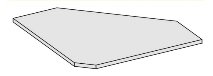
The ESD corner table tops of the Sintro series from Karl meet all the standards prescribed for an ESD-compliant workplace in an EPA to ensure safe working with sensitive electronic components. The surface is slightly structured and glare-free. The volume-conducting carrier plate is resistant to organic solvents, weak acids and alkalis, petrol and oil.
