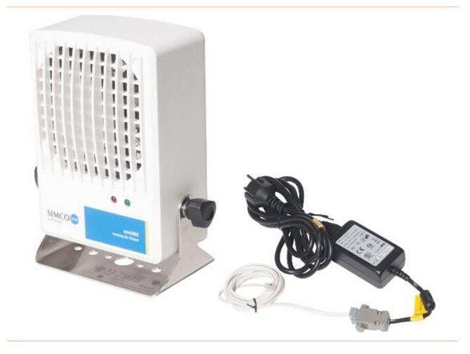
With an ionization device from SIMCO, electrostatic charges can be neutralized at workplaces and in the ESD service area. The integrated blower is infinitely adjustable. In the ionizing unit, the ionization is based on high-frequency alternating voltage (HF-AC).
