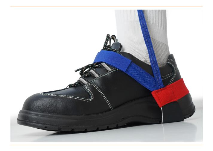
The ESD heel strap from Safeguard is an important accessory for correct personal grounding. It has a leakage resistance of 1 MOhm and a Velcro closure. The heel strap is designed to dissipate static electricity from the feet, preventing damage to electronic equipment and components. The 1 MOhm leakage resistance ensures that static electricity is dissipated effectively and safely. The tape is blue/red and suitable for street shoes with flat heels.
