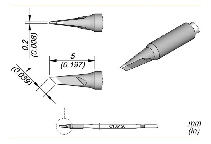
The soldering tips of the C105 series are the smallest tips of the JBC series and are ideal for soldering and repairing very small components. These are compatible with the NT105 and NP105 nano handpieces.
