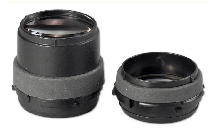
The high-quality Vision Engineering objective MCO-006 with 6x magnification is suitable for use with the eyepiece-free stereo microscope OPTA & Mantis Compact. It can be quickly inserted and removed by simply turning and locking. The working distance is 73 mm, the image section 19.2 mm.
