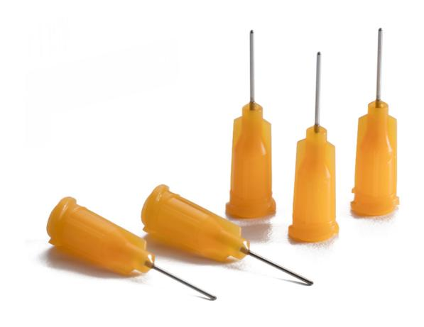
Optimum® beveled tips are perfect for microdot application of low viscosity materials and are manufactured with a special outer diameter cone that reduces wicking for more precise application.
