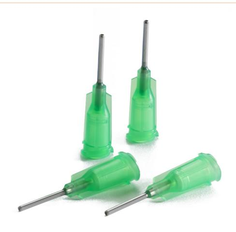
Optimum® beveled tips are perfect for microdot application of low viscosity materials and are manufactured with a special outer diameter cone that reduces wicking for more precise application.
