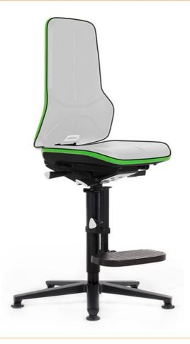
The ESD chair Neon 3 is equipped with five volume-conducting glides and a climbing aid. Its seat height can be adjusted between 590 and 870 mm and features an ergonomics package including permanent contact mechanism. This ensures ergonomic sitting behaviour at your ESD workplace.
