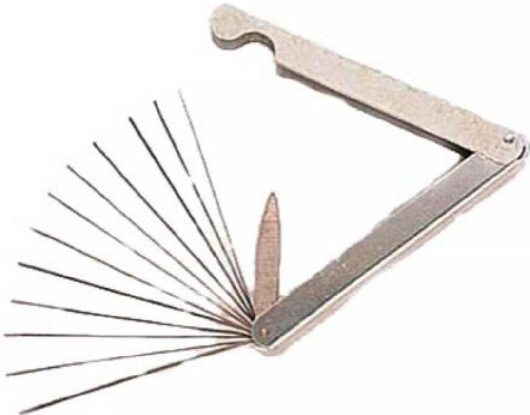
Set of 12 cleaning rods, sizes 0.50 mm - 1.65 mm to remove unwanted solder and flux build-up from desoldering tips. Pack of 12. For use with MX-DS1, CV-H5-DS, and MFR-H5-DS desoldering guns.
