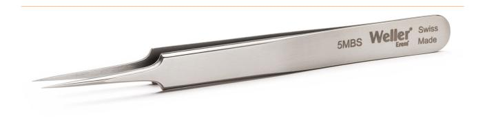
Relieved shape facilitates excellent access to the most confined spaces Special stainless steel, non-magnetic, non-rusting, acid-proof, heat-resistant Heat-resistant up to 500°C (932°F), almost twice as high as Teflon® or Cralon No capillary effect on tips, e.g. while soldering (non-stick property) No contamination caused by positive or negative charge Water-resistant
