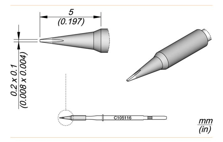
The soldering tips of the C105 series are the smallest tips of the JBC series and are ideal for soldering and repairing very small components. These are compatible with the NT105 and NP105 nano handpieces.
