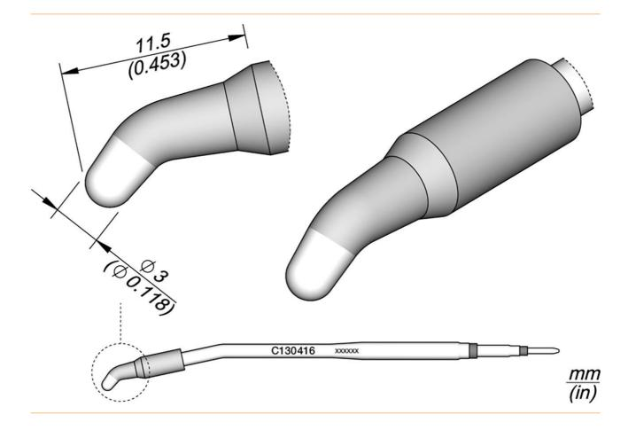
The C130 series of loosening tips are suitable for the AP130 handpiece and have curved tips that are perfectly adapted to the position of the tin wire. The tips can be aligned on the handpiece using the anti-twist device.
