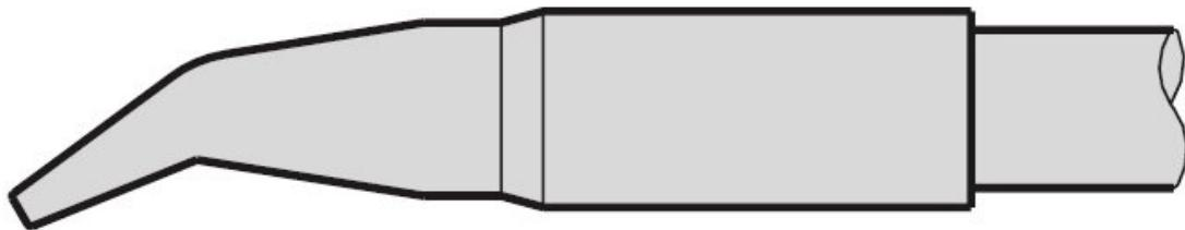
The C130 series of loosening tips are suitable for the AP130 handpiece and have curved tips that are perfectly adapted to the position of the tin wire. The tips can be aligned on the handpiece using the anti-twist device.
