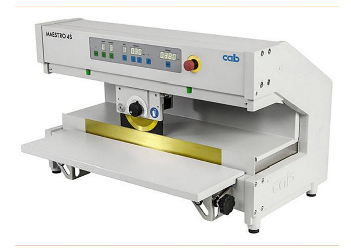
The blade distance is entered on the control panel and adjusted by motor. Up to 9 programs can be set.
