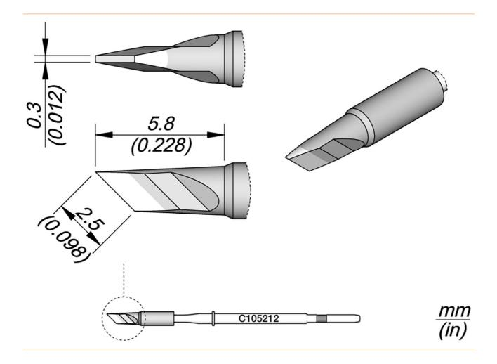
The soldering tips of the C105 series are the smallest tips of the JBC series and are ideal for soldering and repairing very small components. These are compatible with the NT105 and NP105 nano handpieces.
