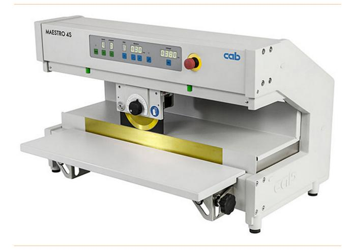
The knife distance is entered on the control panel and adjusted by motor. Up to 9 programs can be set.
