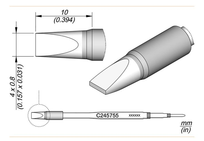
Soldering tips series C245 for soldering iron T245 (formerly AD-2245). They are suitable for general soldering purposes. Sleep and sleep mode in the clipboard. High thermal tip, 40% more efficient heat transfer to the tip
