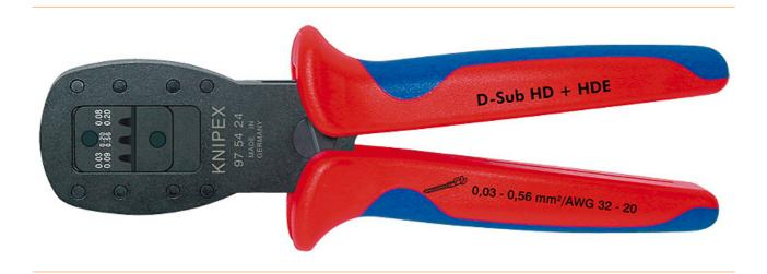
Crimping pliers for miniature connectors Parallel crimp jaws to meet the particularly high demands of small connectors. Consistently high crimp quality due to precision inserts and positive lock (can be unlocked). Crimp pressure is precisely set (calibrated) at the factory, adjustable. Force amplification by knee lever for fatigue-free working. Crimping pliers for other miniature connectors such as HD 22; Modu IV; Micro Timer; ... on request. -
