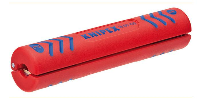
Stripping tool for coaxial cables For stripping and stripping all common coaxial cables from  $\emptyset$  4.8 to 7.5 mm (e.g.: for TV and satellite reception), also suitable for PVC-Flex 3 x 0.75 mm<sup>2</sup>. With length scale 5.0 to 20.0 mm. Double-sided, hinged stripping tool. With opening spring and ratchet. - Cable type: coaxial cable 4.8 - 7.5 round cable 3 x 0.75 mm<sup>2</sup>
