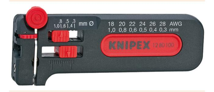
Precise stripping due to gradual adjustment of the tool to the conductor diameter. With wire cutter. With length stop: adjustable from 4.0 to 15.0 mm. With ratchet. For thin copper conductors Ø 0.3 to 1.0 mm. - Stripping values (diameter): Ø 0.3 - 1mm - AWG: 28 - 18
