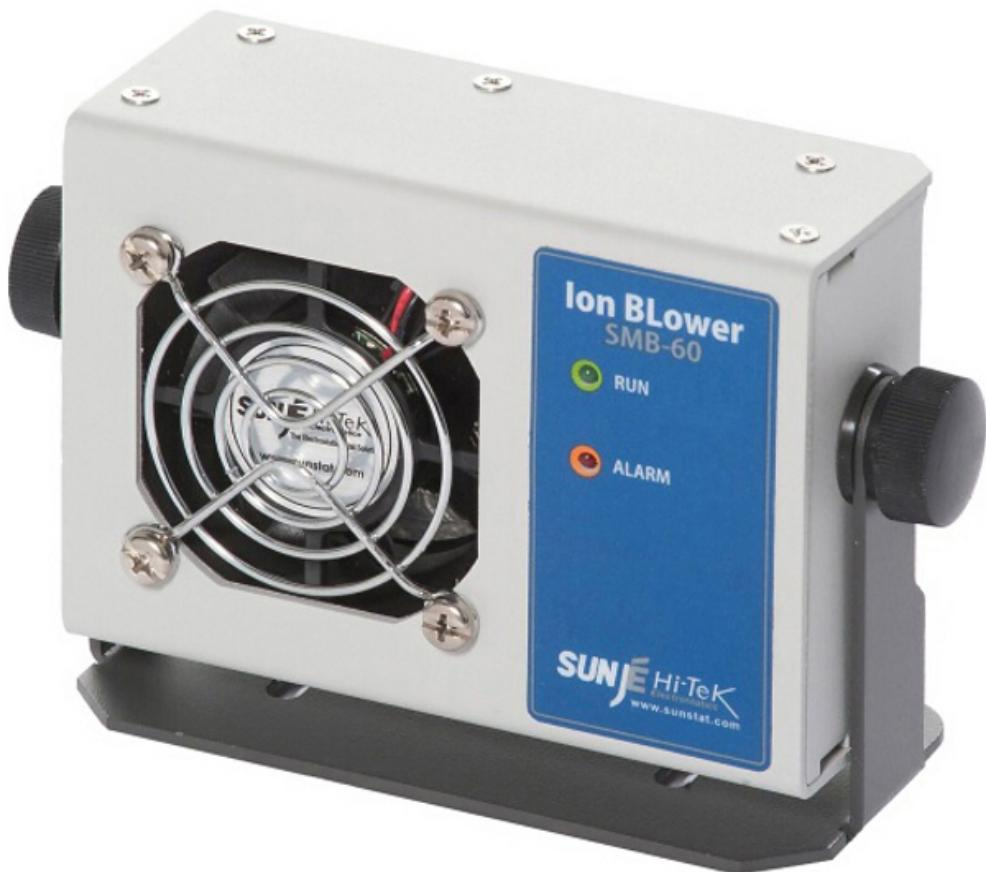
The mobile, small SMB60 ionization unit from SIMCO neutralizes electrostatic charges at workstations and in the ESD service area. The integrated blower is infinitely adjustable. In the ionizing unit, the ionization is based on high-frequency alternating voltage (HF-AC).
