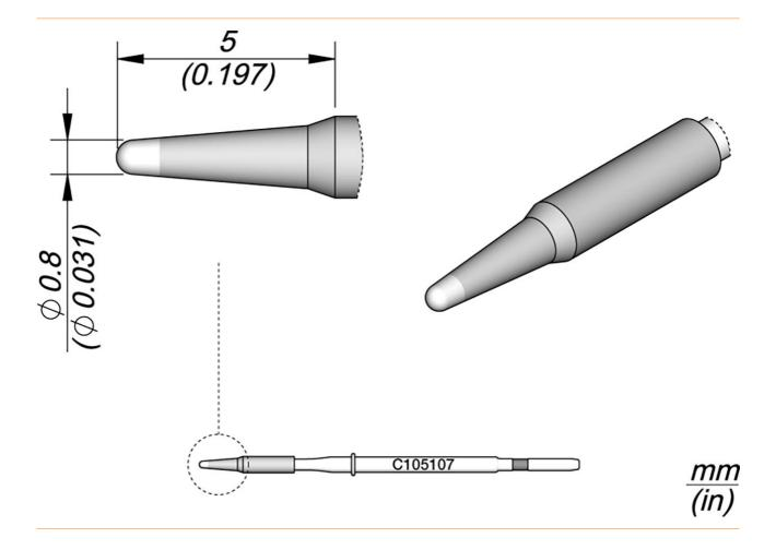
The soldering tips of the C105 series are the smallest tips of the JBC series and are ideal for soldering and repairing very small components. These are compatible with the NT105 and NP105 nano handpieces.
