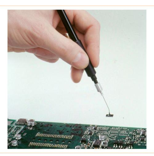
Stand-alone vacuum pick-up system used for pick and place functions. Requires shop air or can be air powered through TS350 Series or TS500R dispensers/controllers. Features an adjustable vacuum control knob to set desired vacuum. Maximum operating pressure 100psi (6.9bar).
