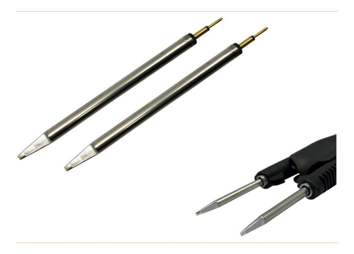
TxP-Tweezer Tip Cartridges are the standard tweezer tip range for the Metcal MFR-series soldering systems. TFP-Tweezer tips are nominally 390 °C. Metcal recommends the TFP-series for most applications. The TCP Tweezer tips are nominally 450 °C and recommended for high temperature and thermally demanding applications. Can be used with leaded and lead-free solder. The Metcal "SmartHeat®-Technology" adjusts power levels automatically based on the demand of the application.
