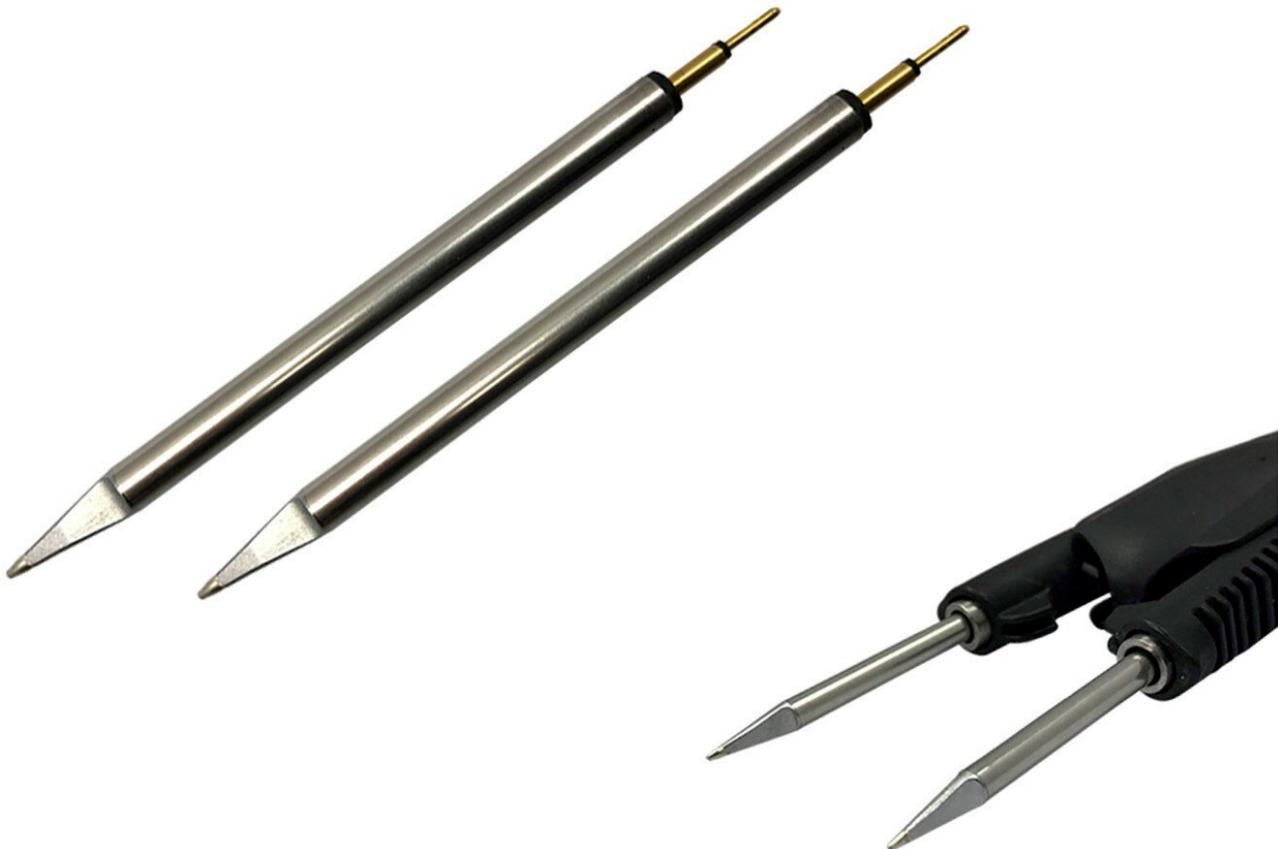
TxP-Tweezer Tip Cartridges are the standard tweezer tip range for the Metcal MFR-series soldering systems. TFP-Tweezer tips are nominally 390 °C. Metcal recommends the TFP-series for most applications. The TCP Tweezer tips are nominally 450 °C and recommended for high temperature and thermally demanding applications. Can be used with leaded and lead-free solder. The Metcal "SmartHeat®-Technology" adjusts power levels automatically based on the demand of the application.
