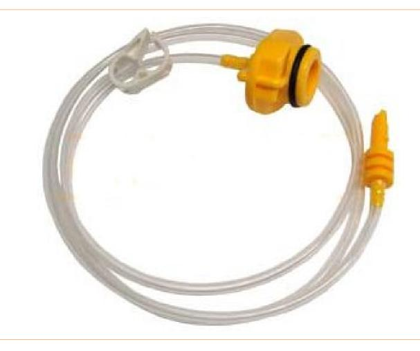
Cartridge adapters are the connection between the controller and the cartridge. Connecting hoses are available in lengths of 0.90 m and 1.80 m. The set consists of cartridge adapter, O-ring, hose and quick-release coupling. The cartridge adapters are made of Delrin.
