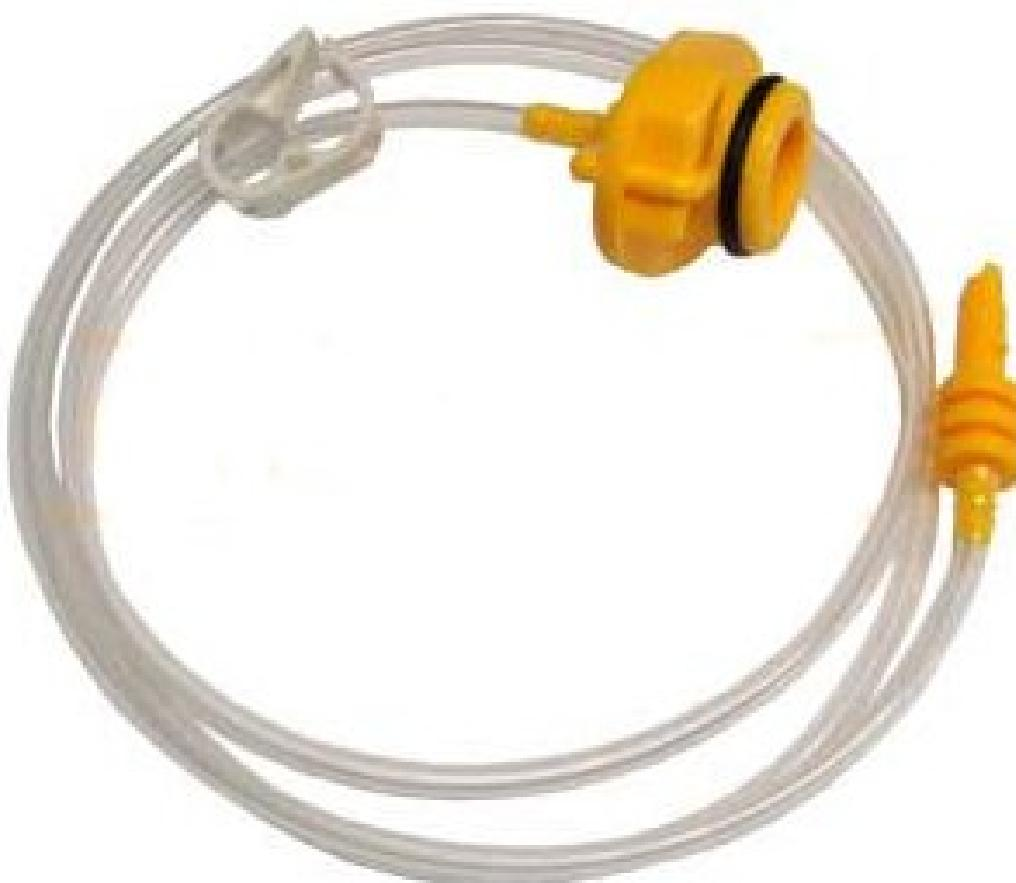
Cartridge adapters are the connector between the controller and the cartridge. Connecting hoses are available in lengths of 0.90 m and 1.80 m. The set consists of cartridge adapter, O-ring, hose and quick-release coupling. The cartridge adapters are made of Delrin.
