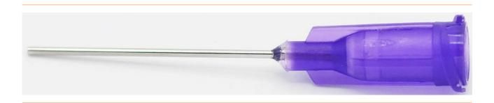
The TE series needles consist of a silicone- and chloride-free polypropylene body with a double helix thread and a stainless steel cannula. The dosing needles are burr-free and have electrolytically polished cannulas that guarantee a constant material flow. Available in packaging units of 50 pieces.
