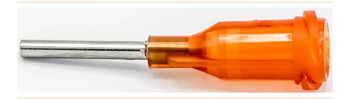
The dispensing needle 1/2", straight, GA 15, amber from Nordson EFD offers outstanding performance for precise material applications. These TE series needles consist of a silicone and chloride-free polypropylene body with a double helix thread and a stainless steel cannula. With electrolytically polished needles for consistent material flow, they are ideal for a variety of assembly applications. Available in packs of 50.
