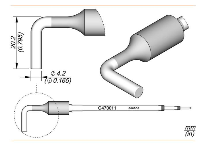
for use up to 500 °C with supply unit HDE (formerly HD-4700) Length of angled piece: 20.2 mm
