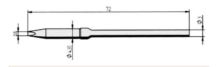
Continuous soldering tip with ERSADUR-LF coating with increased service life
