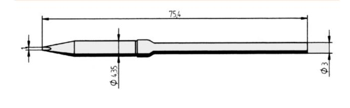
Continuous soldering tip with ERSADUR-LF coating with increased service life
