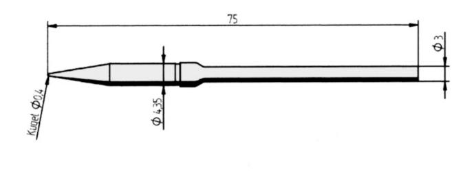
Continuous soldering tip with ERSADUR-LF coating with increased service life
