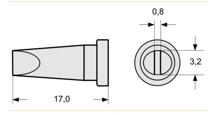
with anti-twist protection for use in automatic soldering machines - together with radiator HER
