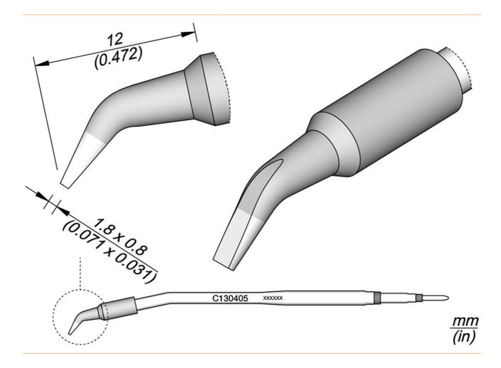
The C130 series of loosening tips are suitable for the AP130 handpiece and have curved tips that are perfectly adapted to the position of the tin wire. The tips can be aligned on the handpiece using the anti-twist device.
