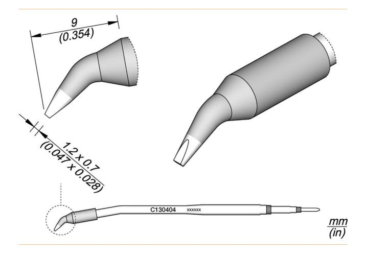
The C130 series of loosening tips are suitable for the AP130 handpiece and have curved tips that are perfectly adapted to the position of the tin wire. The tips can be aligned on the handpiece using the anti-twist device.
