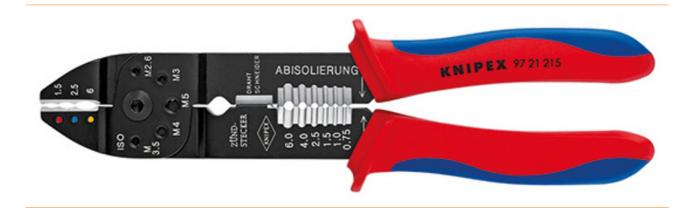
For cutting cables, stripping wires and crimping insulated and uninsulated cable lugs and connectors and open connectors With threaded holes for cutting Cu or Ms threaded pins with M 2.6; M 3; M 3.5; M 4 and M 5. Screwed joint for high stability and smooth running. - Application: insulated cable lugs + cable connectors - Capacity square millimetres: 0.5 - 6.0mm<sup>2</sup> - Number of nests: 3 - AWG: 20 - 10
