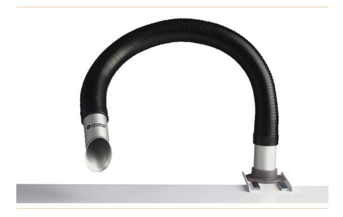
The Alsident System 50 Flex is intended for an air volume of 45 - 85 m3/h and has a pipe diameter of 50 mm. The Flex system is particularly suitable for the electronics industry and laboratories.
