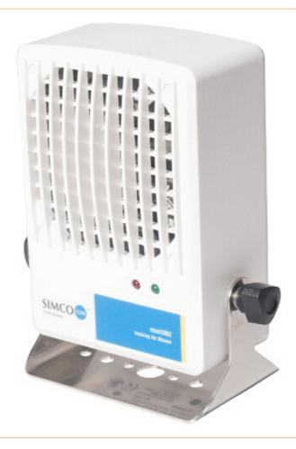
With an ionization device from SIMCO, electrostatic charges can be neutralized at workplaces and in the ESD service area. The integrated blower is infinitely adjustable. In the ionizing unit, the ionization is based on high-frequency alternating voltage (HF-AC).
